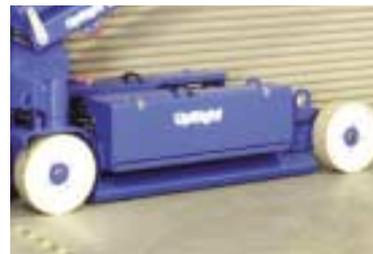
Hydraulic depression mechanism system activates when platform is elevated.
